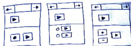
Figure 4: All contain a page navigation bar (top), an audio label (middle) and an interaction element (bottom) – the latter is (from left to right) an audio entry, an audio choice and an audible track bar.
