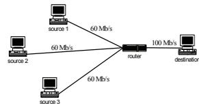
Figure 7: Network topology used for the simulation.
