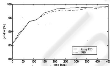
Figure 8: Goodput versus simulation time for both fuzzy PID and conventional PID.
