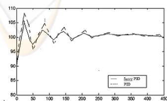
Figure 9: Queue length versus simulation time for both fuzzy PID and conventional PID.
