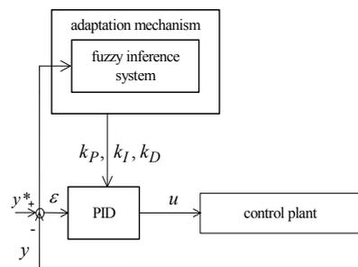
Figure 3: Block diagram of the closed-loop system with adaptation mechanism.
