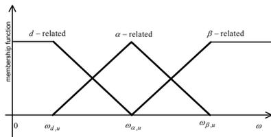
Figure 5: Membership function of the linguistic representing the damped natural frequency  $\omega$ .
