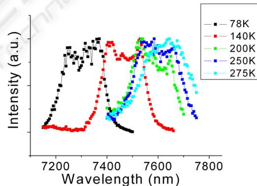
Figure 6: QCL Spectra between 78K and 275K.
