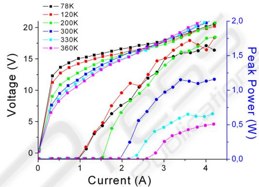
Figure 5: I-V curves and peak power of QCL of our set of laser in the range between 77K and 360K.
