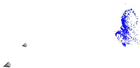
Figure 1: Initial views (gray) and structure (blue) of a human head scene. View positions and orientations are illustrated using pyramid glyphs.
