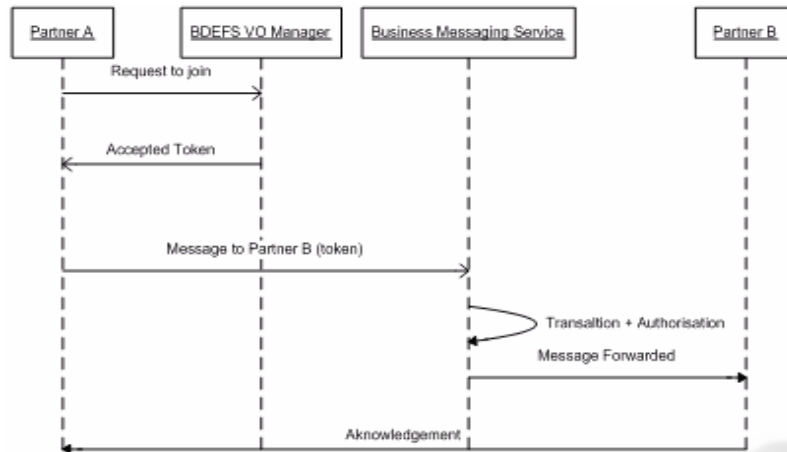
Fig. 2. BDIFS Grid Services Simple Messaging Workflow.
