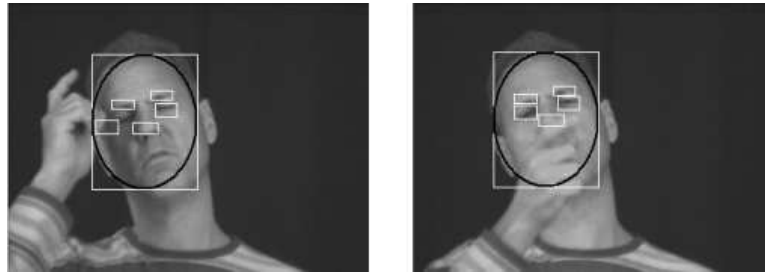
Fig. 2. A template that has been offset due to occlusion (left), and after subsequent recovery (right).
