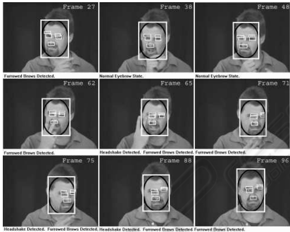
Fig. 3. Selected processed frames from one of the videos. Sign order: JOHN CAR NEVER SEE, English translation: “I have never seen John’s car.” This video has two simultaneous grammatical markers – a headshake and furrowed eyebrows, indicating phrasal negation. Our system detects both of these markers quite well.
