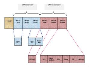
Figure 1: Tag record: UPnP service discovery via a WLAN.
