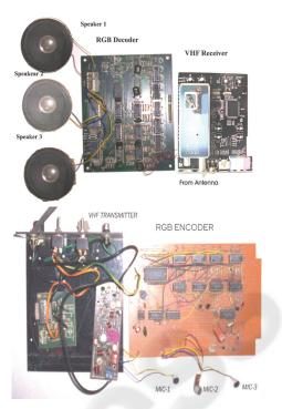
Figure 8: Triple Audio Receiver and Transmitter on Basic Colour Signals (RGB) as carrier signals and built upon PAL VHF Transmitter and Receiver.
