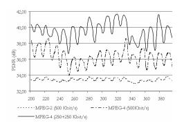
Figure 5: Picture quality obtained after bandwidth adaptation through transcoding.
