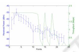
Figure 3: Received power and throughput analysis along path 2.
