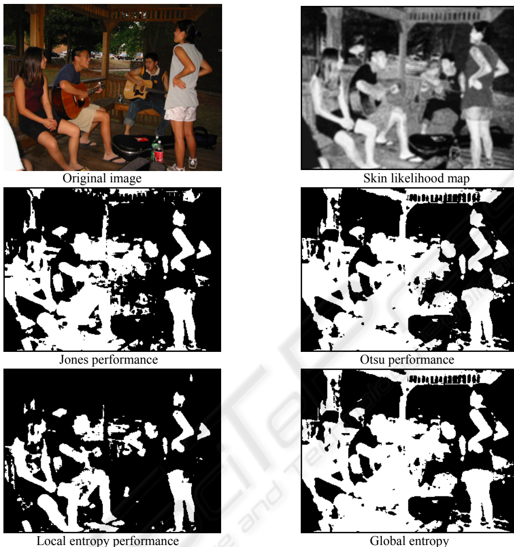
Figure2: The performances of different thresholding strategies on a sample image with a great amount of skin-like background colors.
