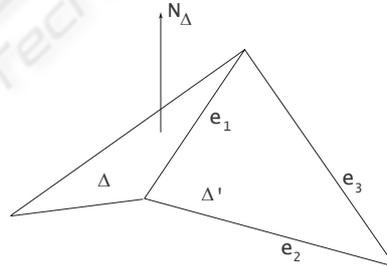
Figure 3: Gehring Compatible Triangles. Here a general projection direction  $N_\Delta$  is depicted.
