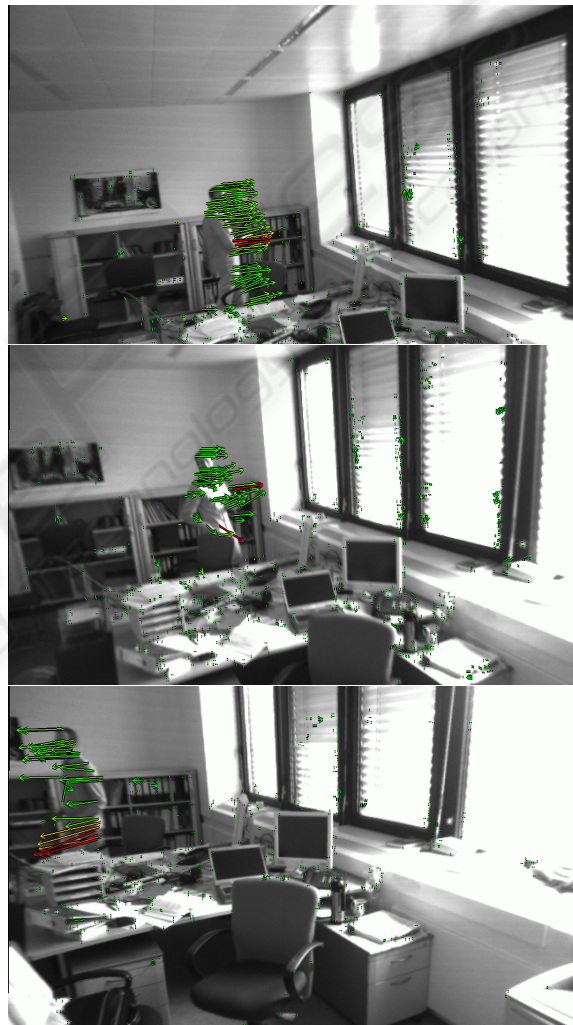
Figure 8: a person moves first to the right (first image), turn around (second image) and finally walk to the left (third image) while the camera is translated and rotated with the hand.
