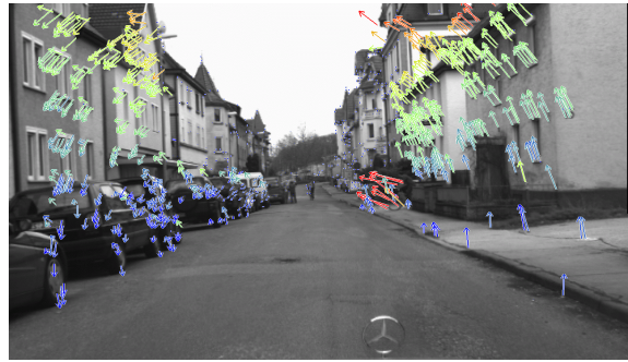
Figure 2: 3D motion vectors obtained when the vehicle drives on an uneven street. Only yaw-rate and velocity are considered in the ego-motion compensation.
