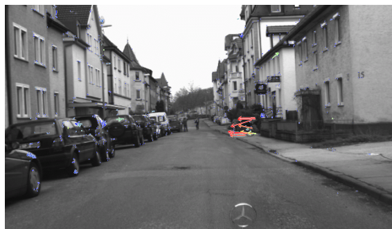
(a) 3D motion vectors. The arrows correspond to the estimated 3D position of the points in 0.5 seconds back projected into the image. The color encodes the velocity as shown in image (c)
