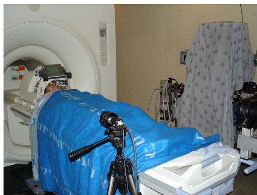
Figure 2: The system configuration. The subject is wearing the device on his head and the two cameras monitor the movements of the tracking device.
