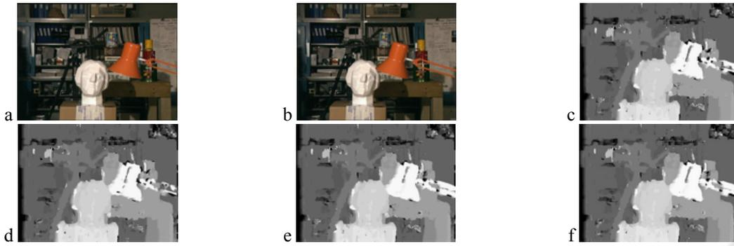
Figure 3: Disparity maps for Tsukuba, block size 8x8 (a) left image, (b) right image, (c) disparity map, M\_SAD, false matches: 19,62%, (d) disparity map, RGB\_1\_SAD, false matches: 19,09%, (e) disparity map, YCrCb\_1\_SAD, false matches: 19,3%, (f) disparity map, RGB\_DST, false matches: 18,92%.
