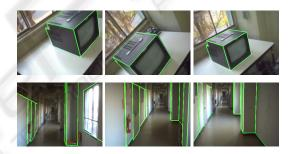
Figure 4: Projected CAD model using tracking results (Top:CRT display[1000frames sequence], Bottom:corridor scene[300frames sequence]).
