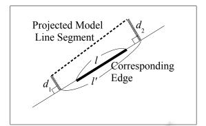
Figure 2: Distance and overlapping ratio between a 3D model line segment and corresponding straight edge.
