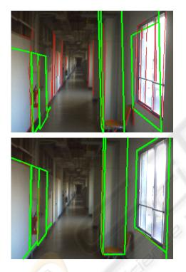
Figure 3: Initial pose and correspondence estimation (Top : Initial guess of the pose and candidates for the corresponding edges, Bottom : Accurately estimated pose and edges corresponding to the line segments of CAD model.
