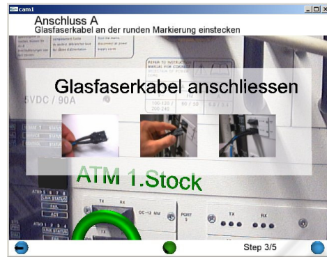
Figure 4: Augmented view, showing additional information how to plug in a connector.
