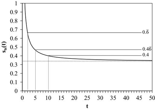
Figure 8: Efficiency of triangle strips in comparison to render each triangle of the strip separately.
