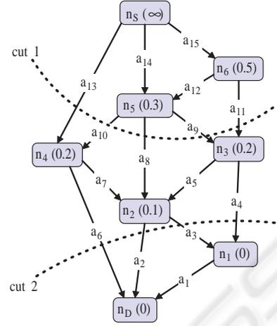
Figure 2: Demonstration of two cuts specifying different LOD. The first cut  $\mathcal{C}_1 = \{a_8, a_9, a_{10}, a_{11}, a_{13}\}$  for  $\varepsilon = 0.25$  and the second cut  $\mathcal{C}_2 = \{a_2, a_3, a_4, a_6\}$  for  $\varepsilon = 0.05$ .
