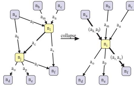
Figure 4: Arc collapse operation: If arc  $a_c = (n_i, n_j)$  is collapsed to a new node other arcs  $a_k, a_l$  and  $a_r, a_s$  are merged to new arcs, that contain larger patches.
