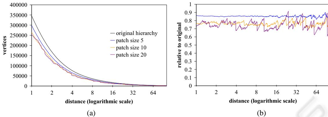
Figure 9: Number of triangle strip vertices of different LOD at different distances using different patch sizes (a) and these numbers of vertices in relation to the original hierarchy (b).
