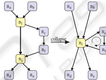
Figure 5: Error situation: If there is another path between two nodes of an arc, this arc can not be collapsed, because a cycle would be created.
