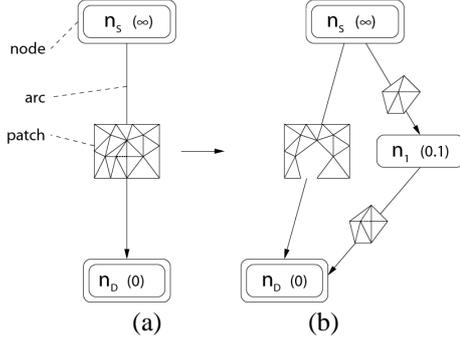
Figure 1: Hierarchy creation steps: basic mesh, the dashed edge is collapsed (a), patch hierarchy after this edge-collapse operation with simplification error 0.1 (b).
