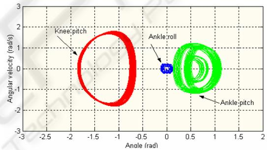
(e) Limit cycles observed in the knee and ankle joints.
