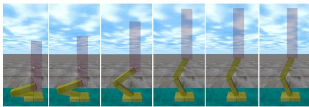
(a) Movement sequence for a fast (400 ms) thrusting the body upwards to assume an upright position.
