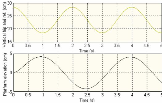
(b) Hip and platform (point of support) positions for a complete cycle.
