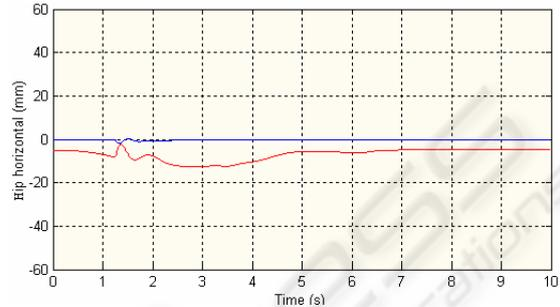
(b) Hip's vertical position under disturbances (left) and hip's horizontal position (right): along the x-axis (in red) and along the y-axis (in blue).
