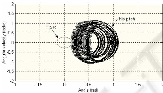
(d) Limit cycles observed in the hip joints.
