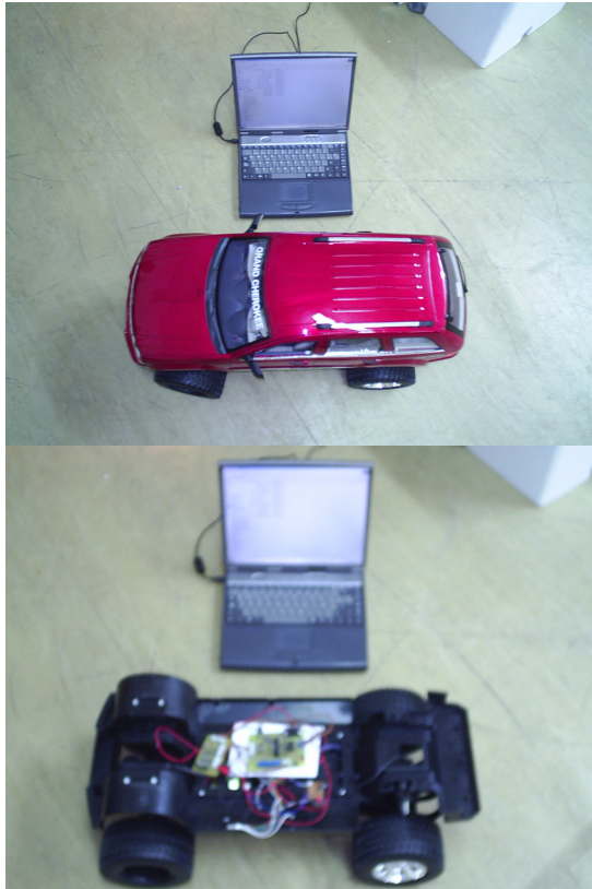
Figure 8: Two sides of the new mobile prototype for platooning guidance used in COVE project.
