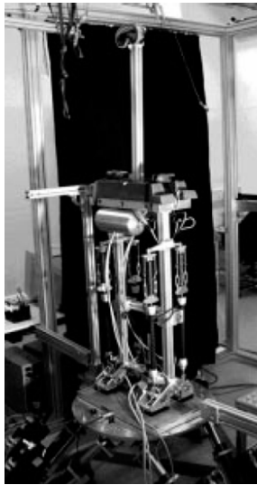
Figure 2: Photograph of humanoid robot ‘PostuRob’ standing on motion platform. Its aluminum skeleton consists of two rigid legs fixed to a pelvic girdle and a spine (‘body’). Center of mass is mainly represented by two plumb weights on pelvis. Each leg carries a front and back ‘muscle’ to move the body with respect to the foot about the ‘foot-ankle’ joint.
