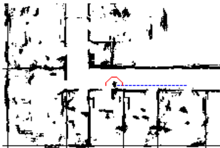
Figure 7: Replanned path (red) returning to the original trajectory (blue, dashed).
