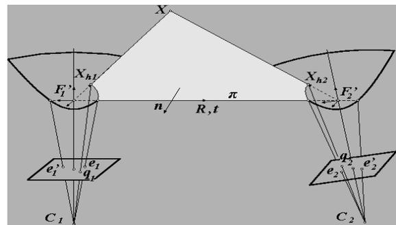
Figure 2: Epipolar geometry for panoramic cameras.
