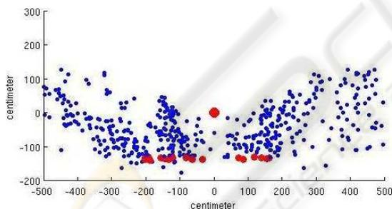
Figure 7: Side view of the 3D-positions of the features. The bigger red dots indicate features on the assumed ground plane.
