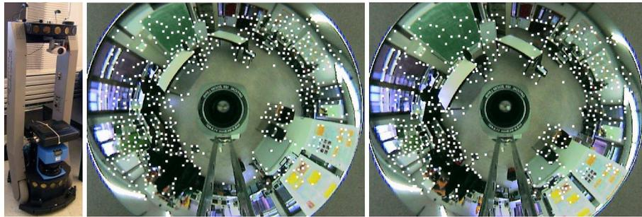
Figure 3: Left: The peoplebot robot. Right: The tracked features in two images with one second delay or fifteen images apart.
