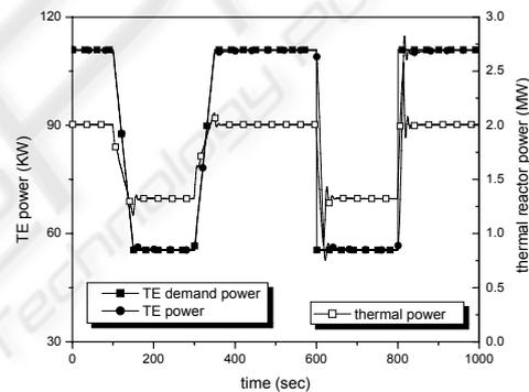
(a) TE power and thermal reactor power
