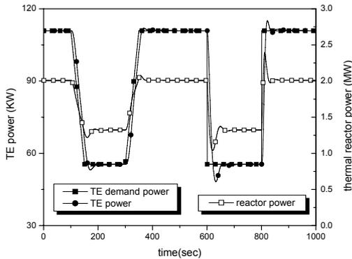
Figure 4: Performance of a PI controller.
