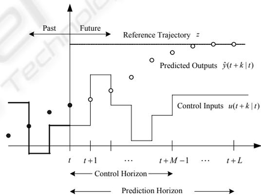
Figure 1: Basic concept of a MPC method.
