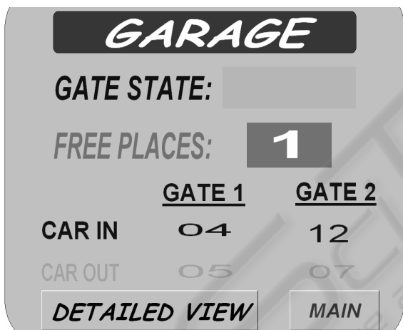
Figure 14: Scada: Park Overview Menu.
