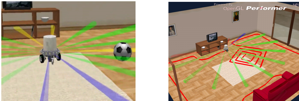
Figure 9: Virtual Prototype: a) General view with a random object; b) Swept area.
