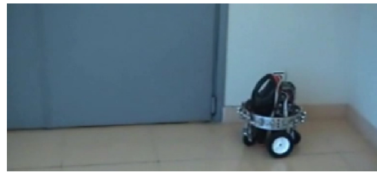
Figure 10: Real Prototype in the wall-following task.
