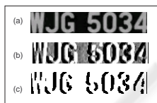
Figure 3: (a)An image of detected license plate (b) Image analysis using RLSA with a new edge detector and 128 offset value (b) Image after applying RLSA and Thresholding Value 1.
