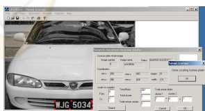
Figure 5: Example of correct license plate detection.
