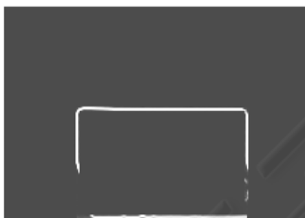
Figure 12: Superimposition of calculated edges on the image of gradient size of a corrupt scan
