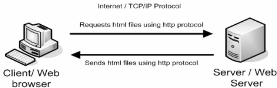
Figure 1: Simplified Client/Server of HTTP communication.
