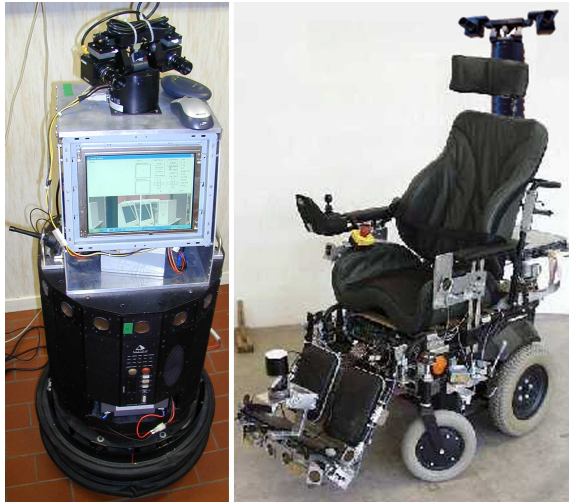
Figure 6: The Nomad200 and wheelchair with the active stereo vision system
