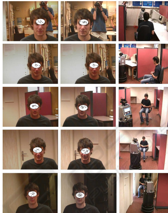
Figure 7: Target tracking results: the white ellipse indicates the goal which is tracked, the small circles represent the different particles of the particle filter. The columns show (1,2) stereo head tracking, (3) robot advancing to the target.
