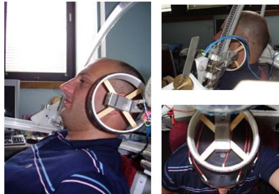
Figure 3: EMF Coil Positioned at Top and Side Head Positions.
