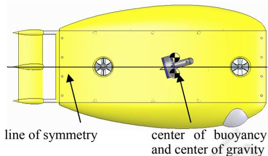
Figure 2: Odyssey IV has highly symmetric thruster placement and a large hydrostatic righting moment
