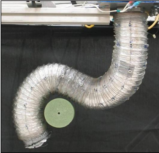
Figure 1: Continuum Robot "Air-Octor."
