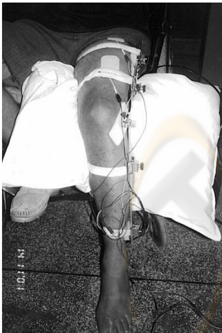
Figure 1: Patient with electrical goniometer to control knee joint
