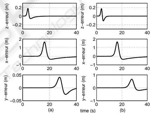
Figure 6: Displacement errors: (a) with axes orientation - (b) without axes orientation.
