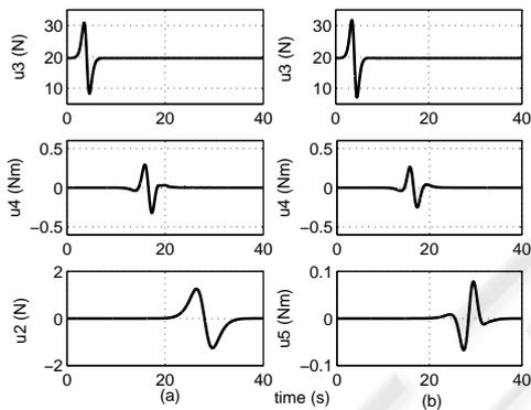
Figure 8: Inputs  $u_2$ ,  $u_3$ ,  $u_4$  and  $u_5$  for the  $xyz$  displacement: (a) with axes orientation - (b) without axes orientation.
