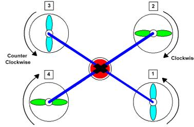
Figure 4: Rotor rotations with yaw motions.
