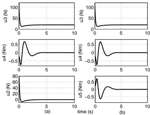
Figure 12: Inputs  $u_2$ ,  $u_3$ ,  $u_4$  and  $u_5$  for the vehicle without motion planning: (a) with axes orientation - (b) without axes orientation.
