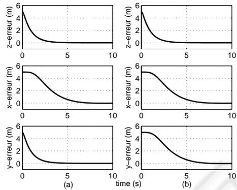
Figure 10: Tracking errors without motion planning ( $z_r = x_r = y_r = 5m$ ): (a) with axes orientation - (b) without axes orientation.
