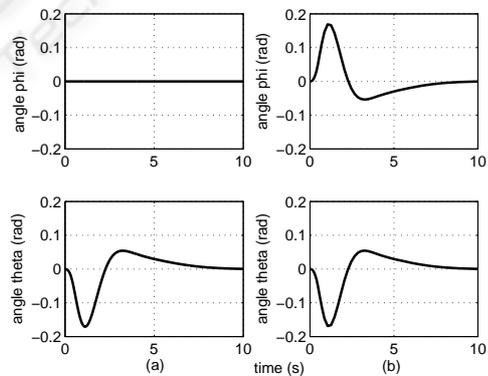
Figure 11: The pitch  $\theta$  and the roll  $\phi$  for the vehicle without motion planning: (a) with axes orientation - (b) without axes orientation.
