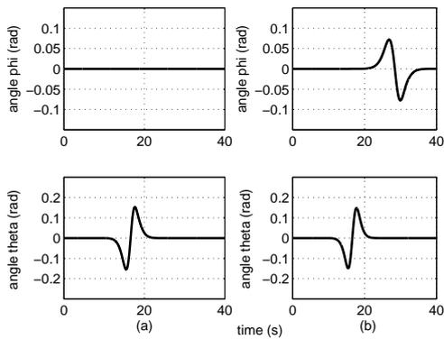
Figure 7: The pitch  $\theta$  and the roll  $\phi$ : (a) with axes orientation - (b) without axes orientation.
